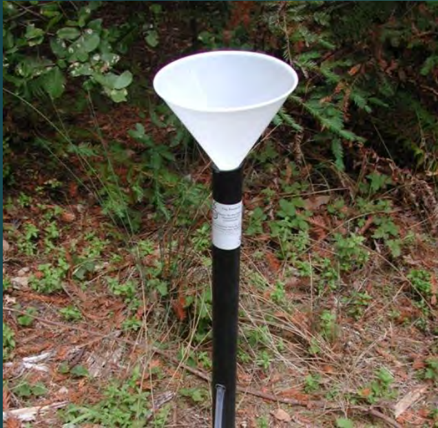
Mixed ion-exchange (IER) resin columns
