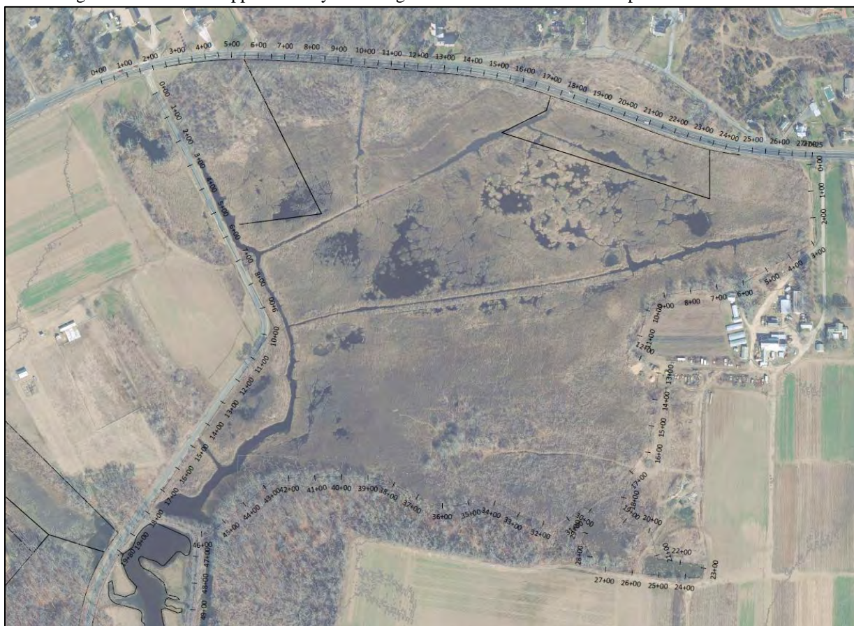
Figure 7: The LiDAR elevation data was evaluated along the edges of the study area with three profiles: 1) Route 25 from W-E; 2) Narrow River Rd from N-S; 3) the eastern and southern property boundary from N-S.
