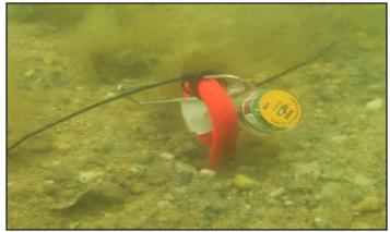
**Figure Intro-1.** A TidBit v2<sup>®</sup> temperature logger attached to a screw anchor, deployed on-site.
