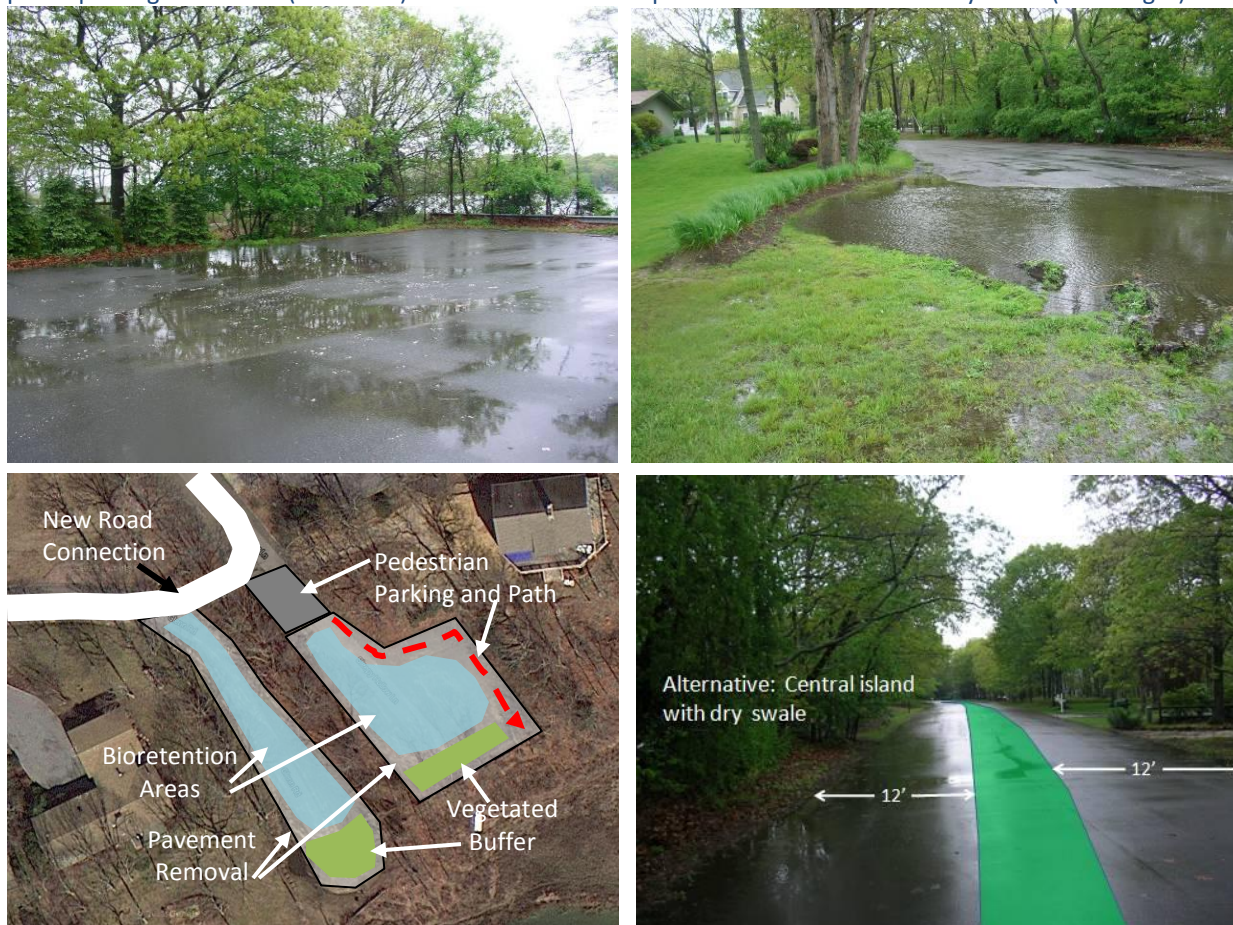
Figure 4.11. Ponding at the end of Sleepy Hollow Lane (upper left) and at the end of Glenn Road (upper right). Proposed concept includes connecting the roads, pavement removal, construction of bioretention areas, and public parking and access (lower left). The additional concept for a central island with dry swale (lower right).
