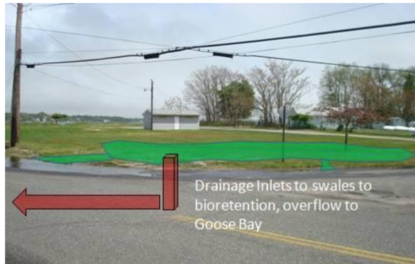
Figure 4.18. Existing conditions along North Bayview Road at the mouth of Goose Creek (top photos). An existing depression within the nearby public park presents an opportunity to repurpose the depression as a bioretention area to improve storage, groundwater recharge, and water quality within the subwatershed (right).
