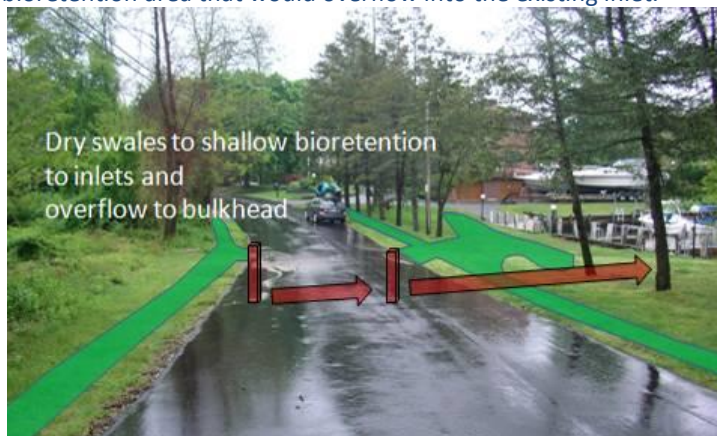
Figure 4.10. Sedimentation along Glenn Road (left). Proposed retrofit (right) would involve construction of dry swales along Glenn Road directed to a shallow bioretention area that would overflow into the existing inlet.
