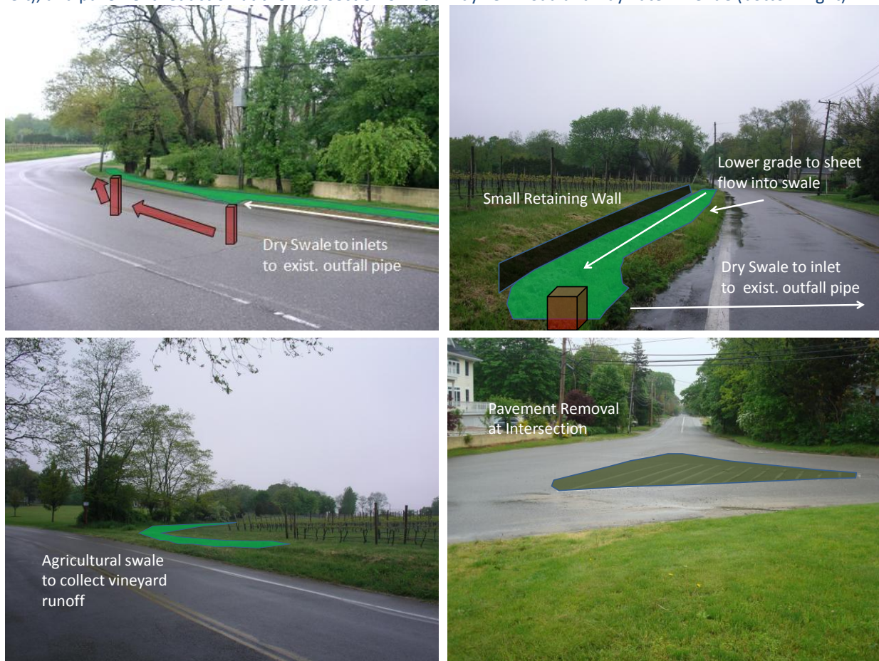
Figure 4.4. Main Bayview Road facing north (top). Proposed dry swales would direct stormwater to the existing outfall pipe at Goose Creek. Proposed BMPs could also include a vegetated swale within the vineyard (bottom left), and pavement reduction at the intersection of Main Bayview Road and Baywater Avenue (bottom right).
